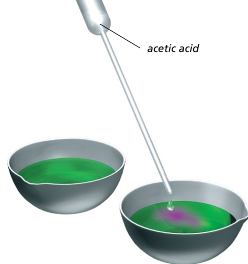
The green potassium manganate decomposes when you add acid, and the purple permanganate returns.
