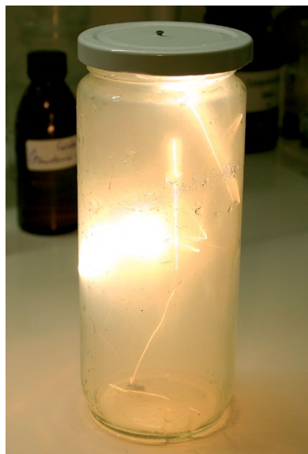
Even an iron wire will burn in pure oxygen.
