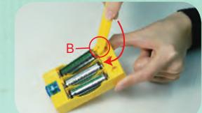
To later remove a battery from the holder, use the "B" end of the part separator tool.
