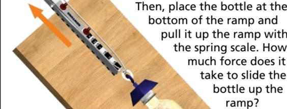
Then, place the bottle at the bottom of the ramp and pull it up the ramp with the spring scale. How much force does it take to slide the bottle up the ramp?
