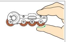
Test that gears move smoothly. If they stick, check if there are burrs left on the gears, and remove them.
