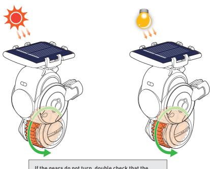
If the gears do not turn, double check that the gears were assembled correctly (page 10).
