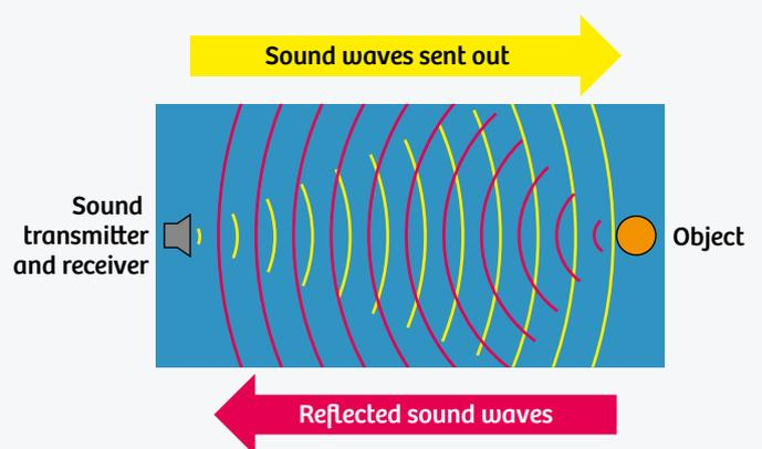
The ultrasonic sensor has one transmitter and one receiver.
