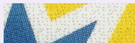
A close-up of a code card showing the OID pattern of dots
