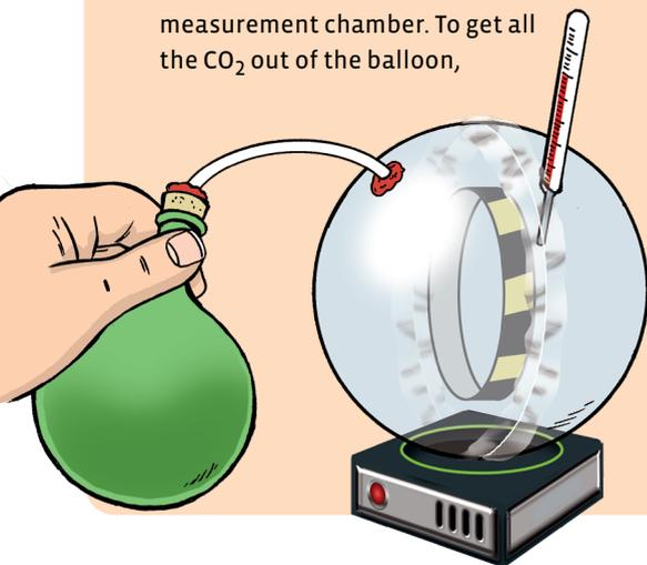
gently squeezing the balloon. Try to keep liquid from getting into the tube. When the balloon is limp and only has liquid in it, pull the end of the tube out of the measurement station and immediately seal the chamber opening with clay.
