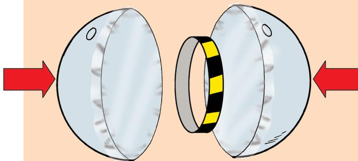
the ends together. Cut two squares of plastic wrap that are about 15 centimeters by 15 centimeters and stretch each square over the mouth of each half-sphere. Set one of the half-spheres in front of you and place the spacer ring in the center of the plastic wrap. Now, fit the two half-spheres firmly together with the spacing strip in between and the measuring holes at the same level, and you will get two separate measuring chambers.
