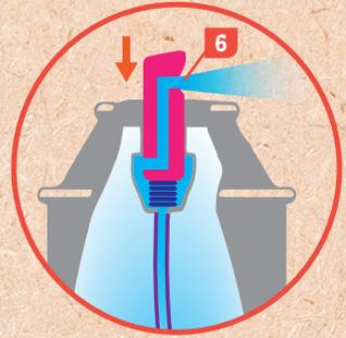
mixture inside the can. When the painter pushes down on the valve, the spring compresses and the channel opens. The high pressure gas wants to push its way out of the can. As it does so, it carries the paint up the dip tube (5) and out the nozzle (6).
