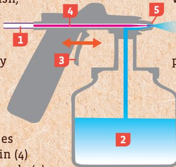
When the nozzle opens, the high-pressure air flows through it. Because of a physical principle called the Venturi effect, this high-speed escaping air creates an area of low pressure at the nozzle which actually sucks the paint right up out of the reservoir!
